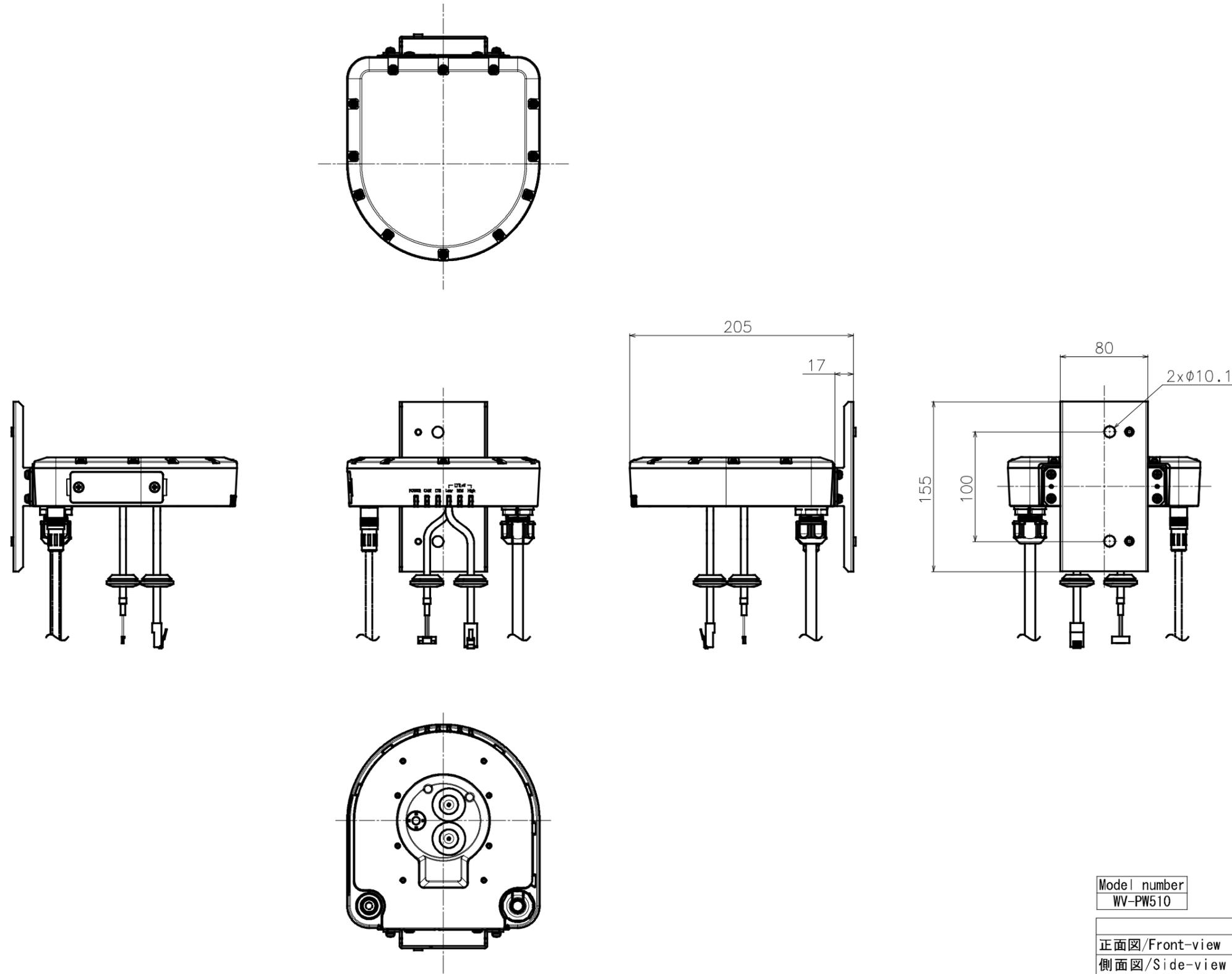
With clamp fixing bracket
