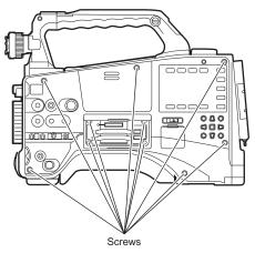
3 Remove the side R panel as shown in the following figure. When removing them, be careful not to put load on the FFC between the main unit and panel and connectors.
