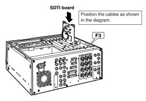
**9** Reattach the board clamp using the screw, then fix the top panel in place using the 2 coin screws.
