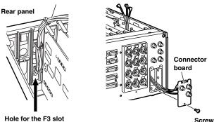
7 Connect the connecting cables to the SDTI board.
