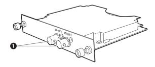
**1)** SDI output connector [SDI OUT1, SDI OUT2] Serial digital component signal can be output.
