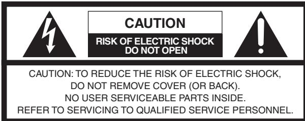
The lightning flash with arrowhead symbol, within an equilateral triangle, is intended to alert the user to the presence of uninsulated "dangerous voltage" within the product's enclosure that may be of sufficient magnitude to constitute a risk of electric shock to persons.
