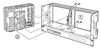
Use the four screws to secure the rear panel and plug the cable of the main controls into the connector on the monitor. (Refer to the instructions in the operation guide of the BT-LH900 series.)
