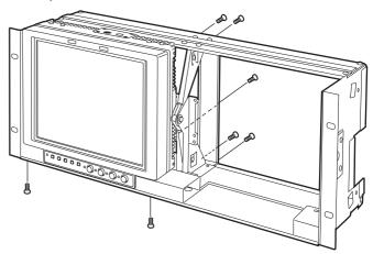
Use the four screws to secure the rear panel.
