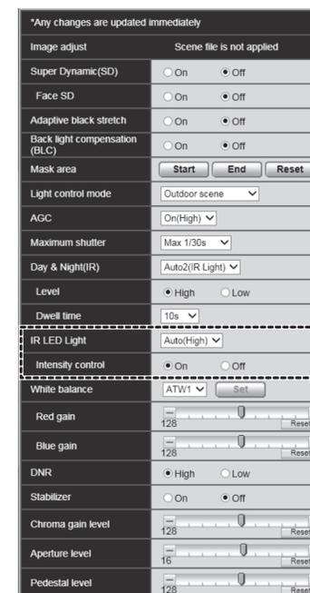
4 When looking at the camera from the front through a digital camera or a smart phone, you can confirm the operating state of the IR LED unit by checking if the point of white light can be seen on the left side of the camera.
