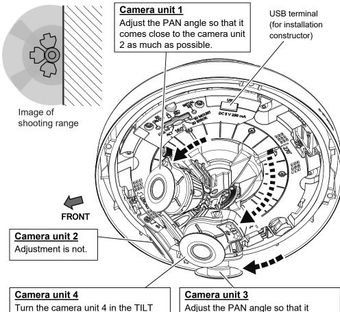
Turn the camera unit 4 in the TILT direction so that it comes into contact with the camera unit 2.
