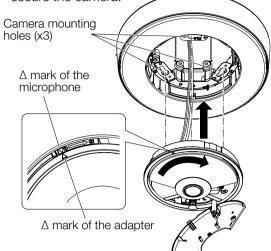
③ Engage the attachment fixing screws in the rear of the camera with the camera mounting holes
