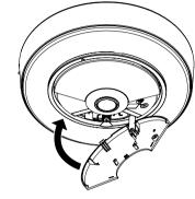
4 Tighten the camera fixing
